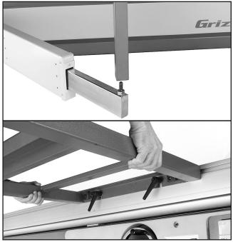
Figure 42. Installing the crosscut table.
